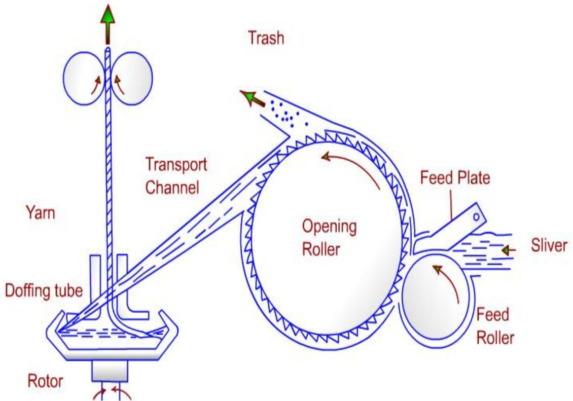
**Main features of rotor spinning system**
