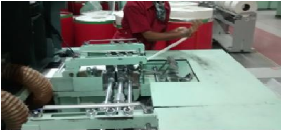
Piecing of sliver to pass through trumpet
