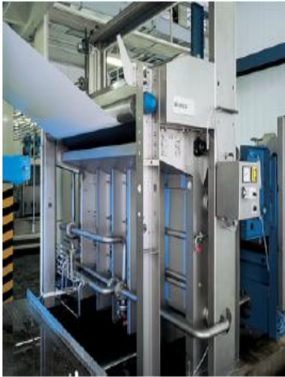
Passage of fabric in chemical trough
