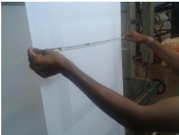
Checking fabric width
