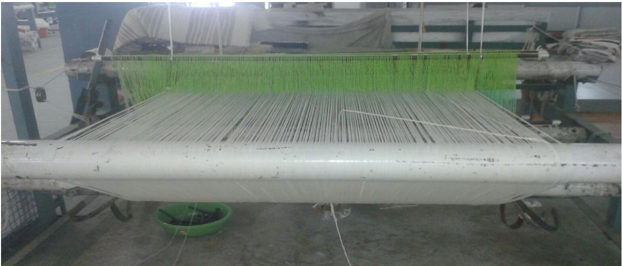
Broken Warp Ends
