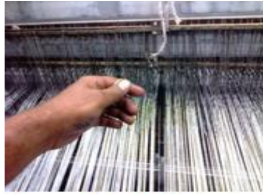
Weaver detects the broken end
