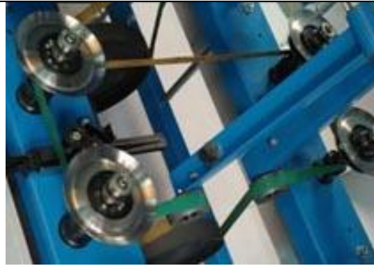
Tape driven four spindle assembly in TFO
