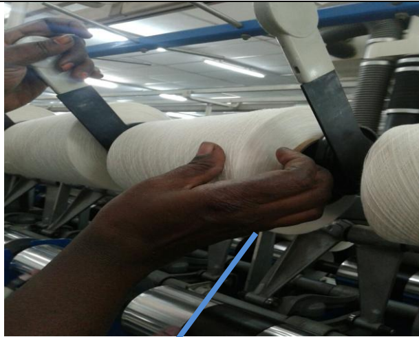
Taking out cone from machine for doffing
