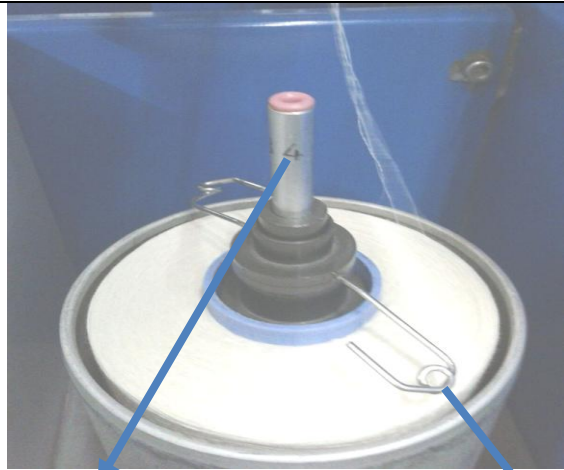
Tension mark on Tension Variator
