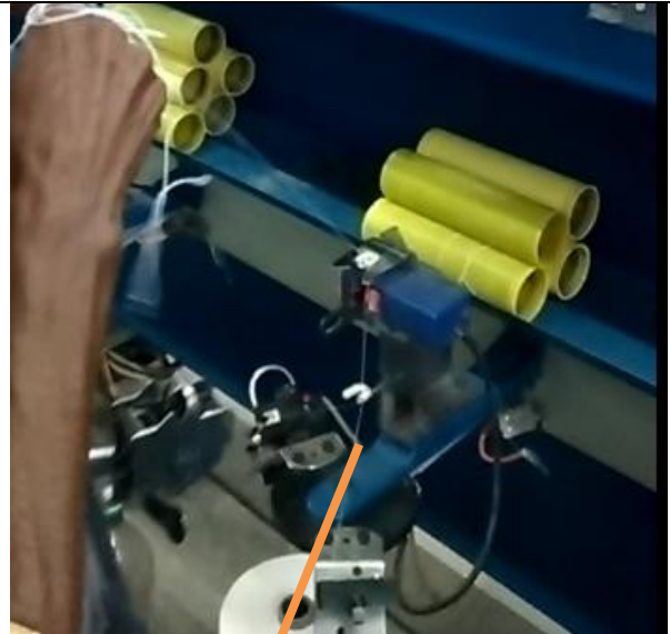
Taking broken thread from cones and passing through tension weight,EYC & thread guides
