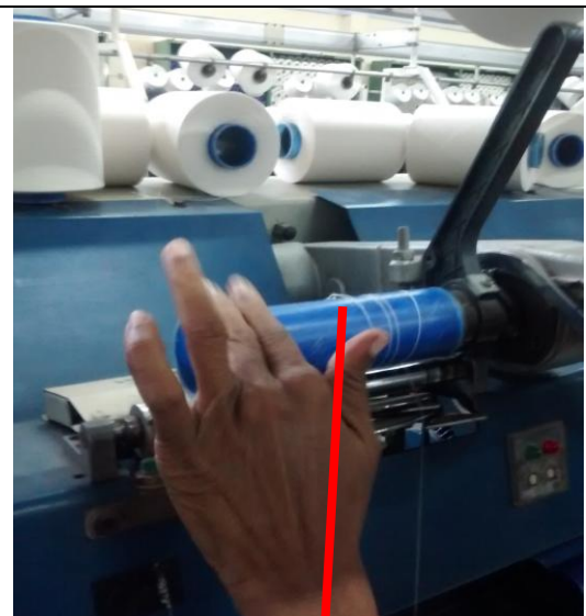
Winding thread on empty cheese
