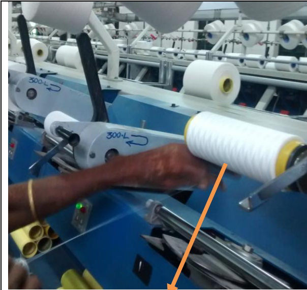
Taking broken thread from cheese
