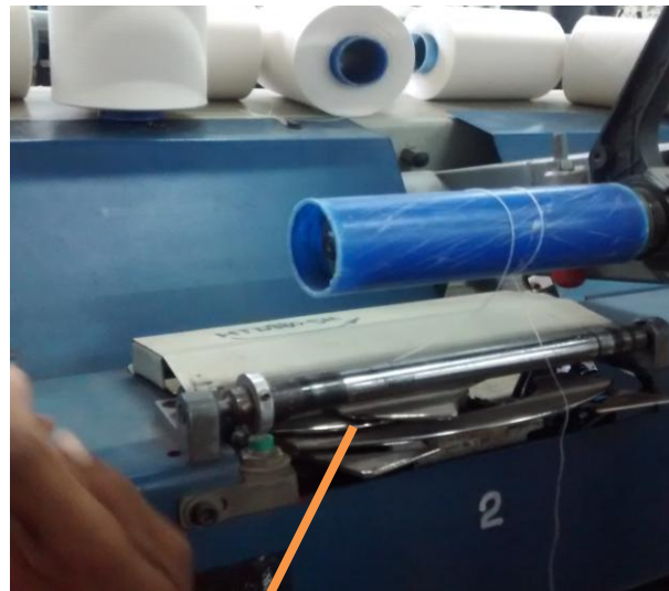
Counter rotating blades for traverse
