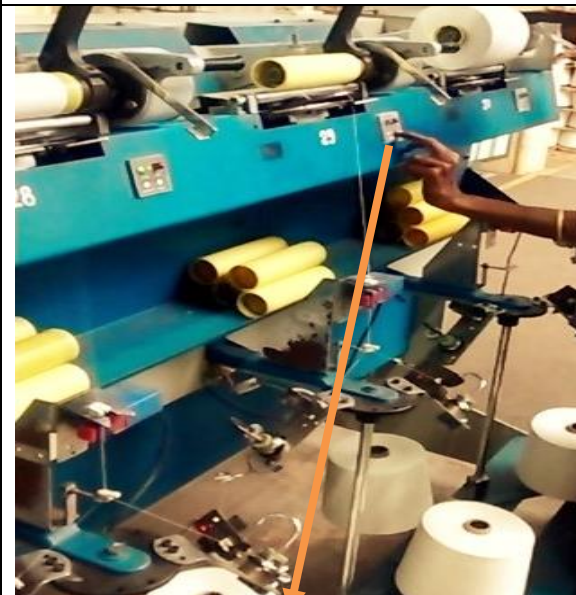
Operating control switches
