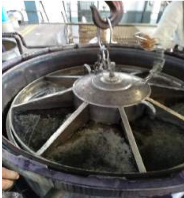
Photo: Dyeing carrier loaded into main vessel
