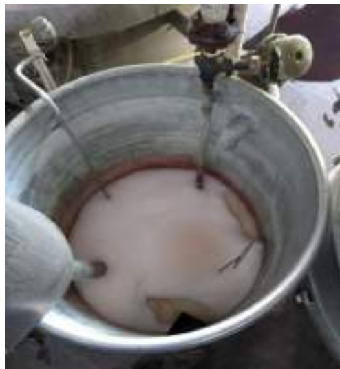
Photo: Colour and Chemical addition tank
