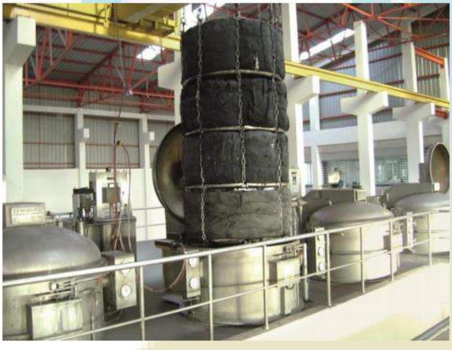
Photo: Loose stock dyeing machine
