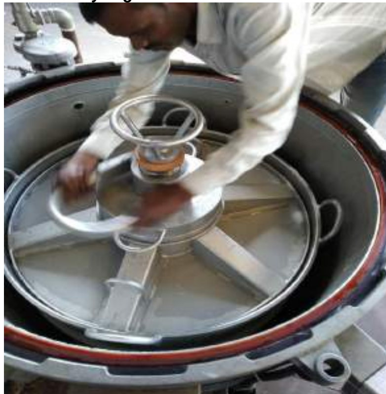
Photo: Fitting of Lid to the dyeing carrier
