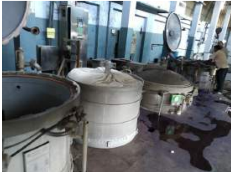
Photo: Dyeing carries and main dyeing vessel
