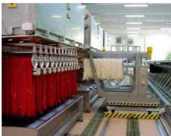
Photo: OBEM automated hank dyeing machine
