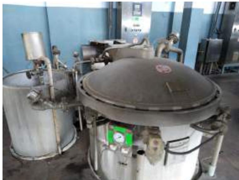
Photo: HTHP dyeing machine ready for dyeing
