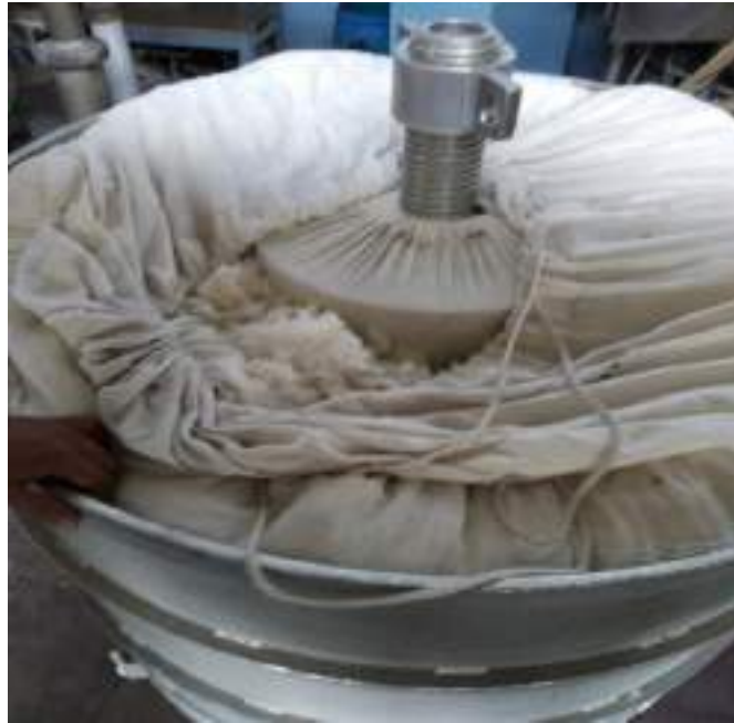
Photo: Perforated carrier with wool fibres loaded
