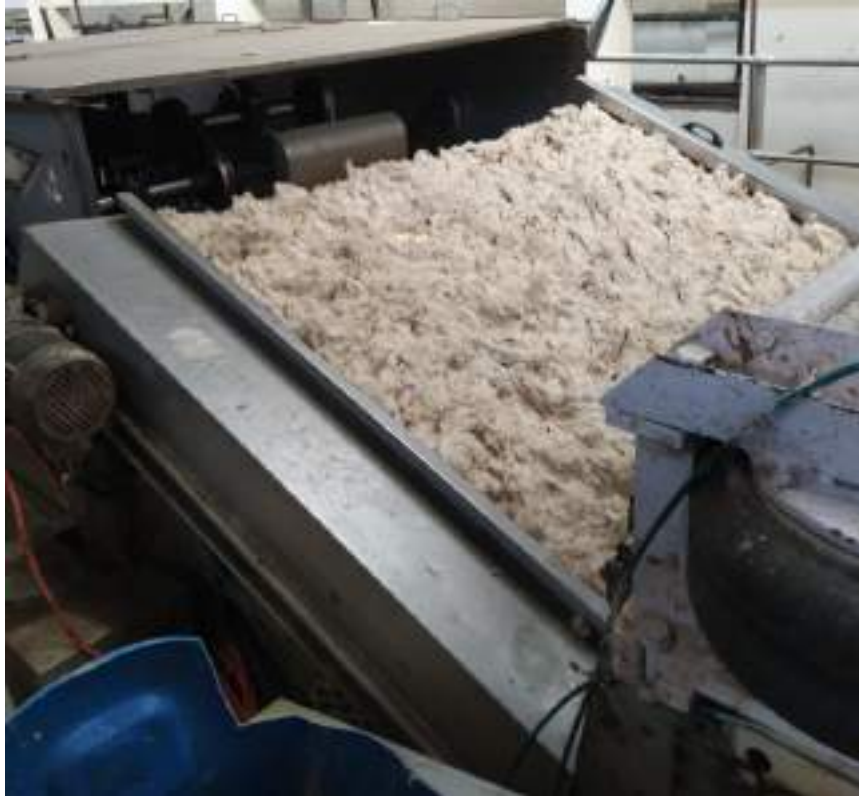
Photo: Wool fibre scouring (after scouring in first Bowl the fibres are squeezed and forwardd to second Bowl)
